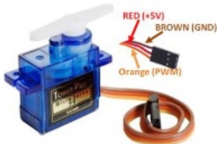
Figura 11. Pinout del servomotor.
