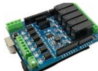
Figura 2. PLC control shield. (Tomada de www.jelelectronica.com )
